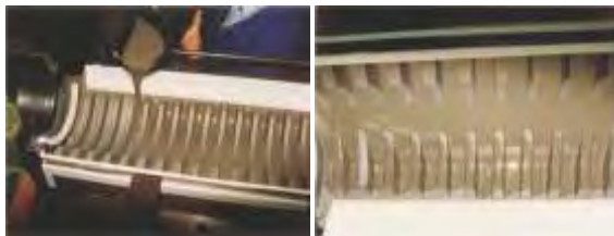
moulding of a hydrostatic tooth rack without machining
