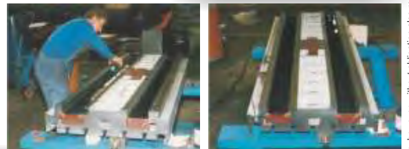
moulding of flat ways by pouring
